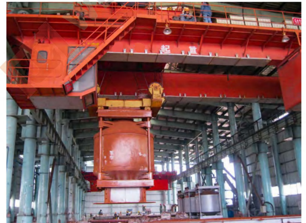
▲ 全自动垃圾焚烧发电起重机 Full-automatic crane for garbage incineration power generation
