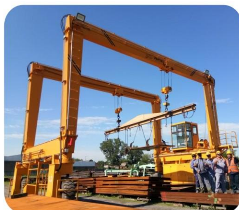
Hydraulic double girder type Capacity: 10t~200t Span: 10-20m Lifting height: 6-15m
