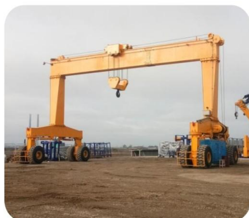
Hydraulic single girder type Capacity: 10t~100t Span: 10-20m Lifting height: 3-12m
