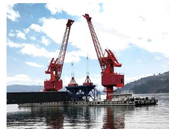
Single Jib Fixed Portal Crane Capacity: 10t~40t Working radius: 10~20m
