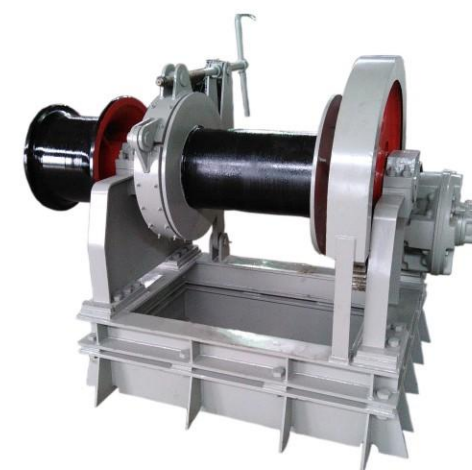
Hydraulic mooring winch Capacity:5t~100t Rope length:1000m Rope speed:9~12m/min
